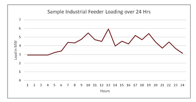
Figure 35: Electrical loading of an industrial feeder (24 hours)
