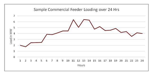
Figure 34: Electrical loading of a commercial feeder (24 hours)
