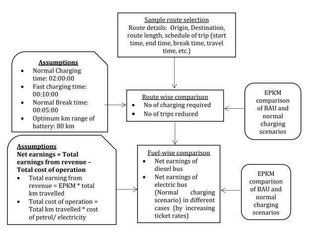
Figure 14: General methodology for the viability study of short-range battery buses \*EPKM, earnings per kilometre
